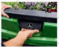
Pick-up style tailgates fold out to 90 degrees and down to a full 150 degrees.
